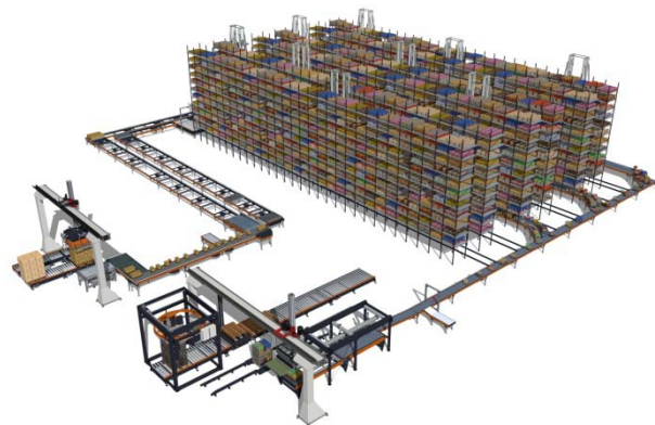
Figure 2 : automated casepicking system (ACP)
