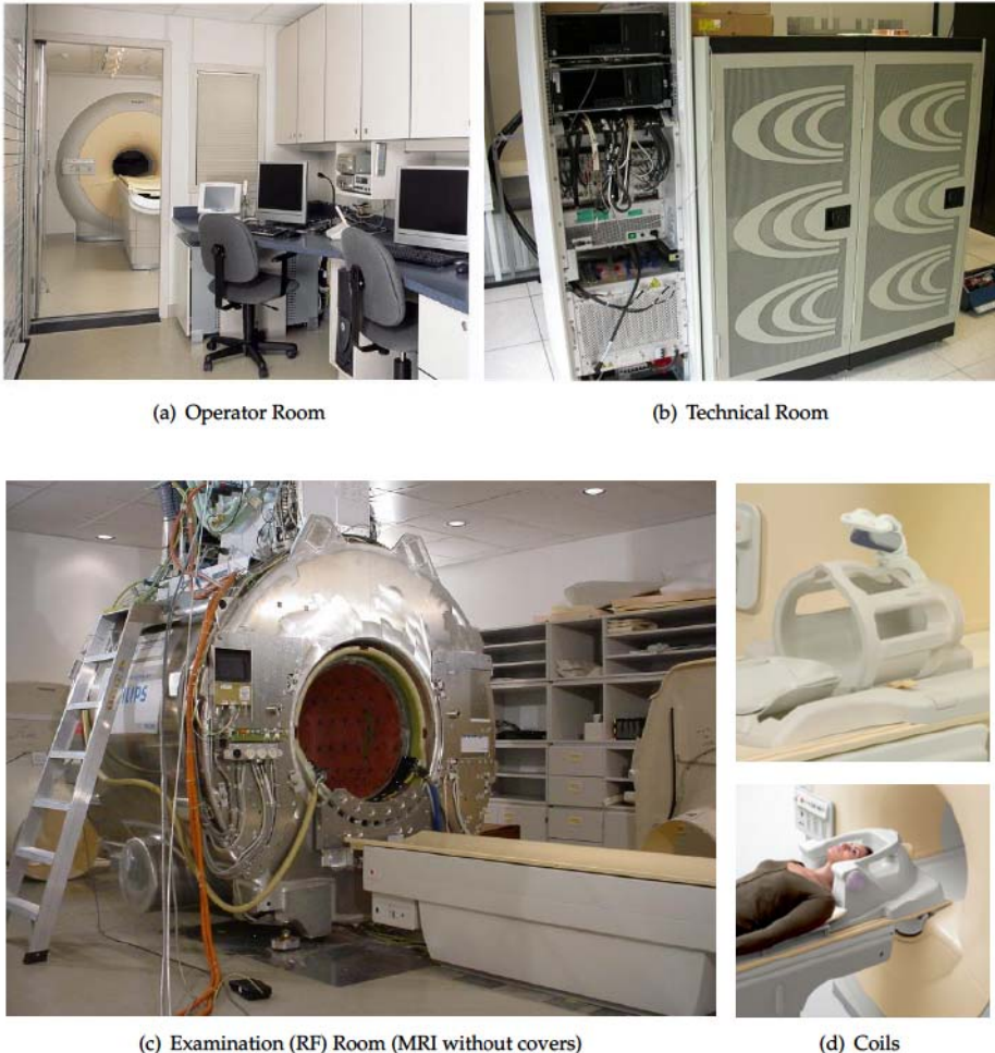
Figure 2.3: Philips MRI System (Courtesy of Philips Healthcare)
