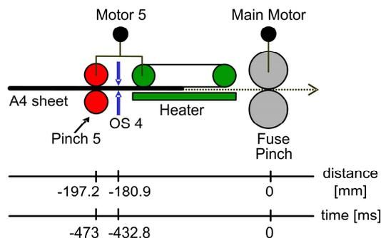
Fig. 3. Schematic representation of Motor 5 and its environment, together with distances and traveling times to the Fuse Pinch
