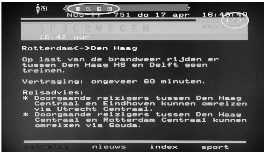
Figure 3.7 Philips television that has combined a page with sub-pages (codes 01, 02, 03) and one without sub-pages (code 00) broadcasted after each other.
