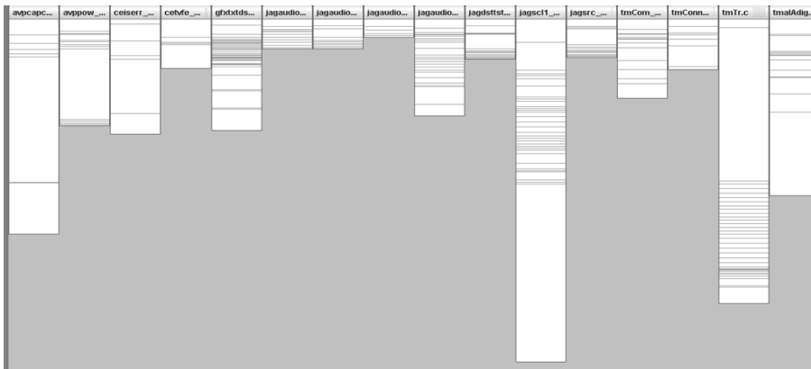
Figure 6.2 The scattering of a concern over multiple files is visualized using AspectBrowser [Griswold, 1999]. Each source file is depicted as a block. Each source line dealing with this concern is grey and horizontal.
