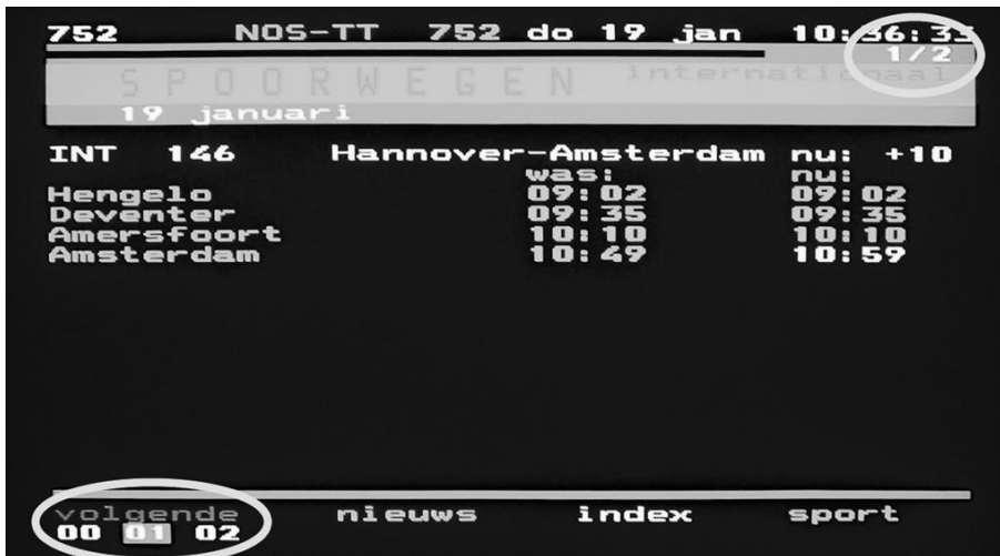
Figure 3.6 Samsung television that has combined a page with sub-pages (codes 01 and 02) and without sub-pages (code 00) broadcasted after each other.
