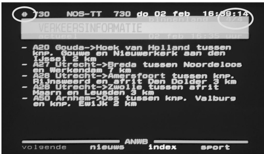
Figure 3.9 Sony television displaying sub-page 4 out of 4, whereas storing out-of-date sub-pages with higher sub-pages numbers (indicated at top left of page by the two arrows signaling the possibility to navigate to sub-pages with lower and higher numbers).
